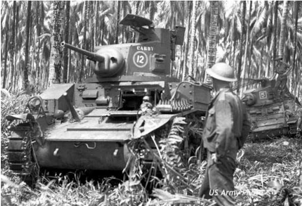
The M3 Stuart Light Tank. While small in size and armament its armor allowed it to advance to effective distance of the Japanese bunkers where its 37-mm gun could engage. 19
